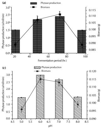
Figure 4: Growth kinetics and phytase production by *Klebsiella pneumoniae* SCTb2: (a) Effect of fermentation period, (b) Effect of temperature and (c) Effect of pH
